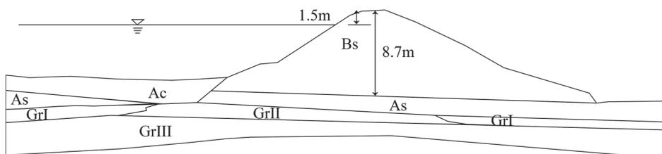
Bs: fill (decomposed granite) Ac: alluvial clay As: alluvial sand
